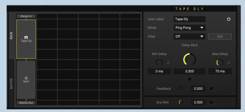
• To change the timing of the doubled voices, you can either pull down **Delay Mod** or push it up. It changes the value from **Min Delay** (in this case 0ms or no delay) to **Max Delay**, (in this case 75ms).
